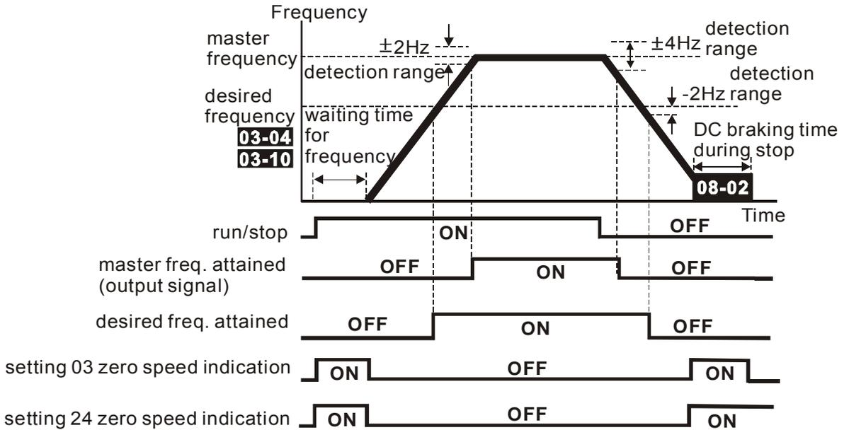
output timing chart of multiple function terminals when setting to frequency attained or zero speed indication
