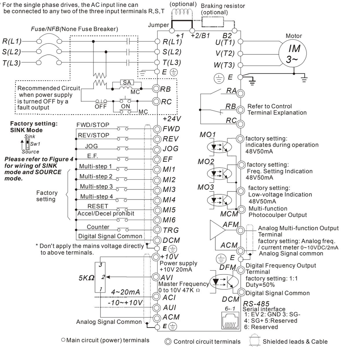
**Figure 2 for models of VFD-B Series**
