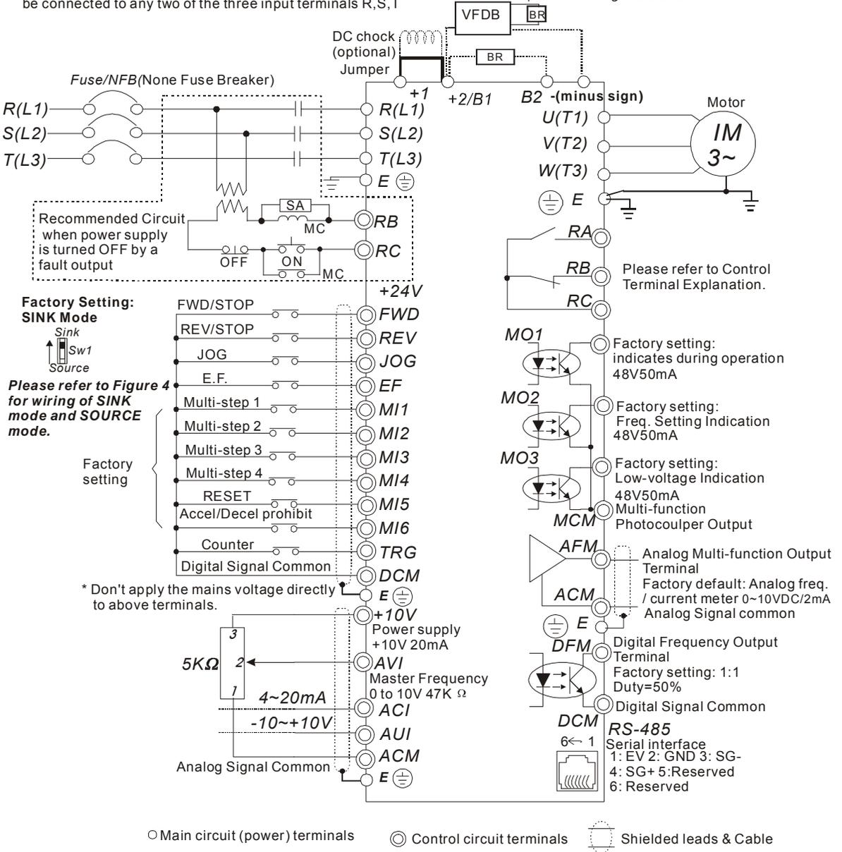
Figure 3 for models of VFD-B Series
